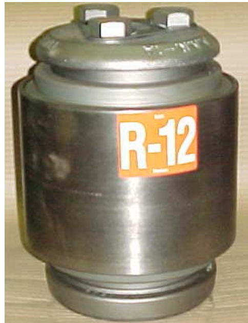
BEARING AFTER RECONDITIONING
